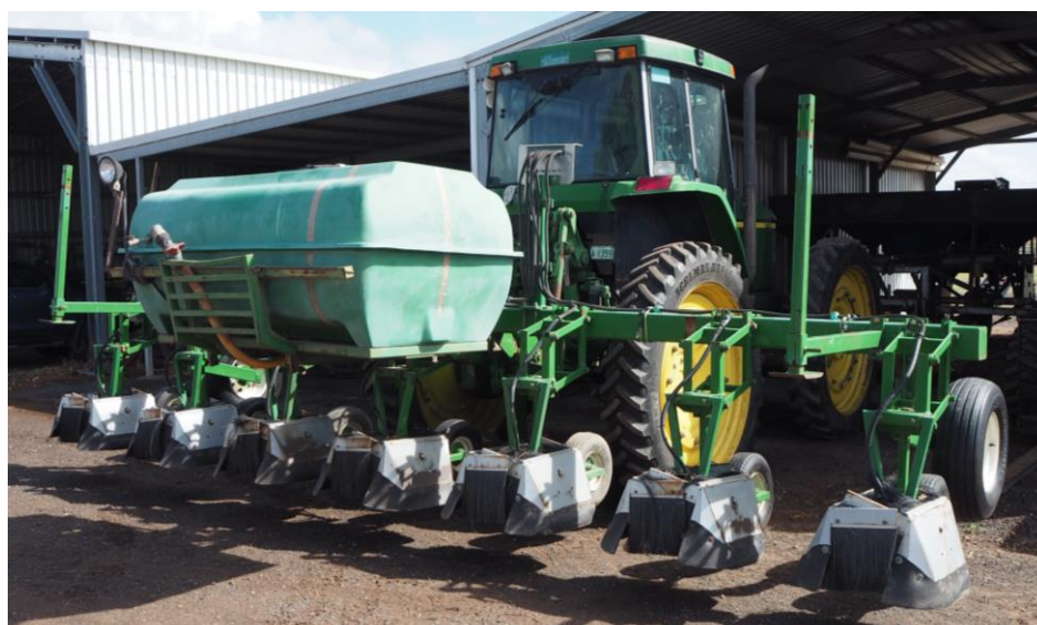
A weed spraying rig with shrouded spray jets to keep weedicide to the interrow and away from the pineapple plants
