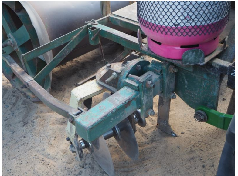
The Telone fumigation rig which hills up at the same time. Matt Stein providing information on fumigants.
