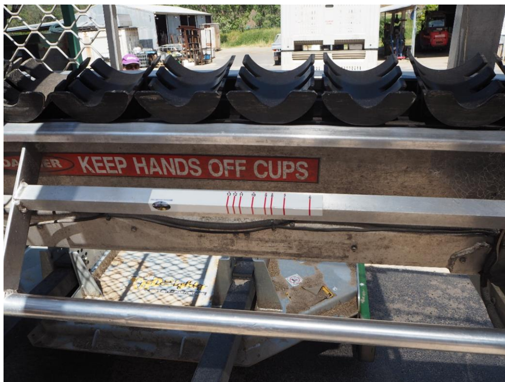
Cannery harvester with de-topper. Stickers with fruit measurements along the boom.
