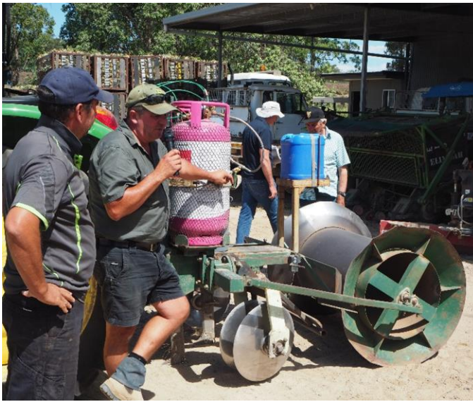
The Telone fumigation rig which hills up at the same time. Matt Stein providing information on fumigants.
