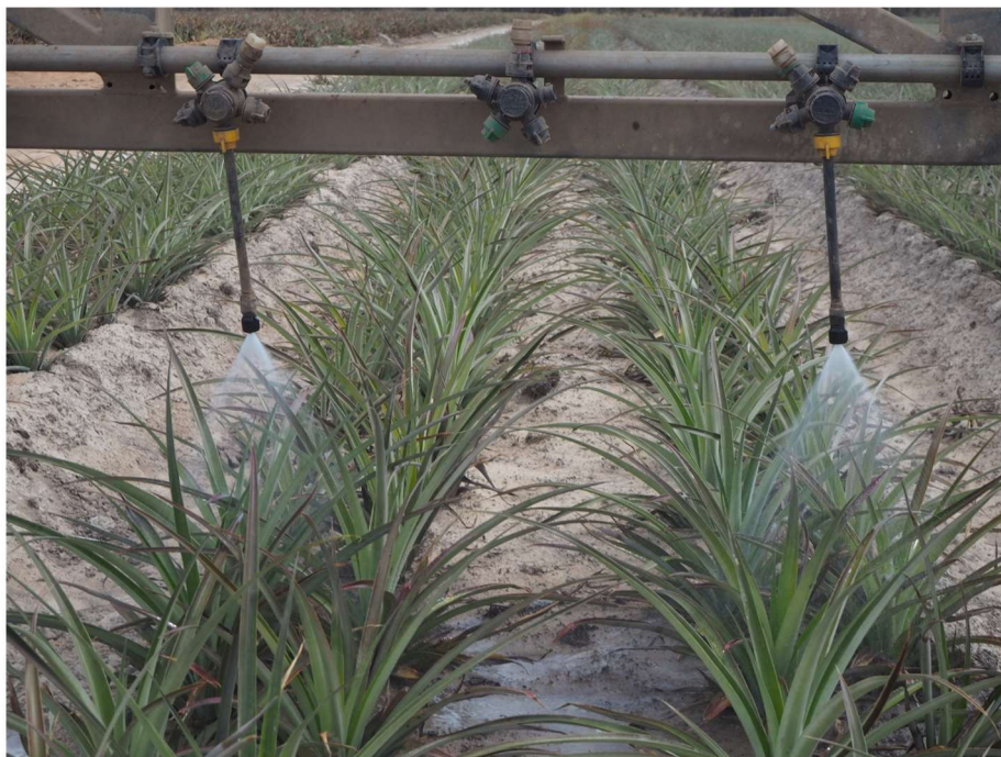
Spray boom droppers target the spray on pineapple plants only, achieving chemical savings and benefits for the environment
