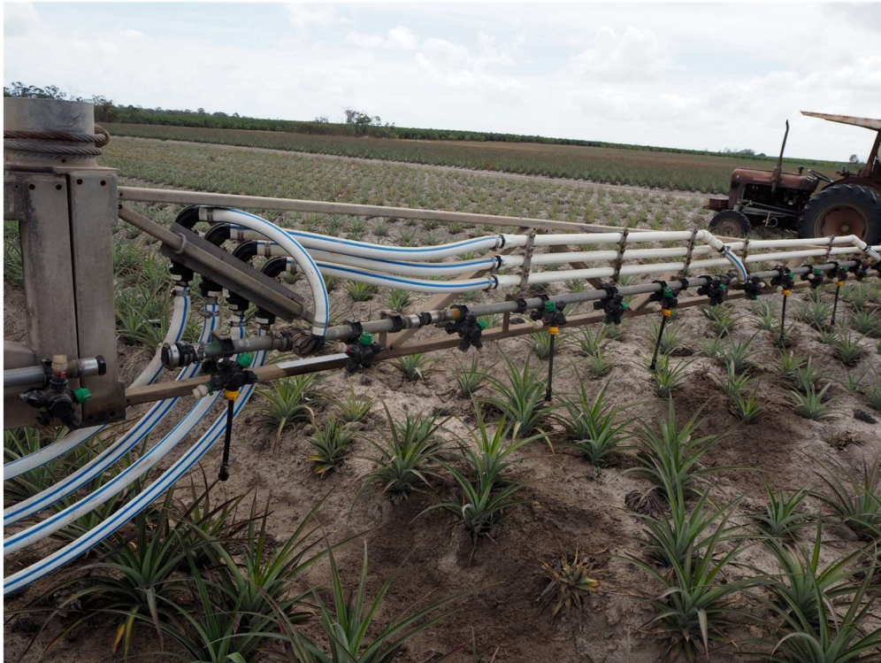
Variable rate spray boom showing some of the variable rate sections. Eventually these sections will be controlled by GPS. The folding point of the boom is visible on the left.
