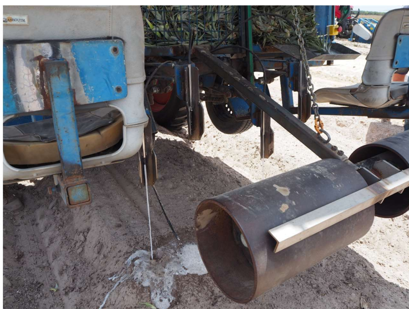
The planter injects a shot of water (and potentially chemical) into the planting hole as the top or slip is planted. Here the planter has been raised to show the water jet in action. Inclusion of the rollers also saves a second tractor operation. The water tank is mounted on the front of the tractor.
