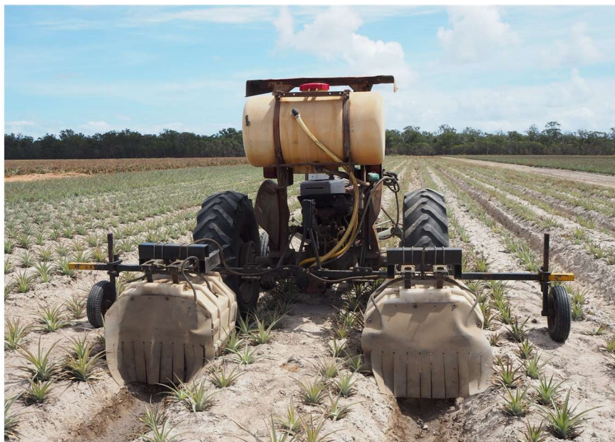
The Hubert's rig which confines weedicide to the interrows and protects the pineapples from chemical spray by using shrouds around the jets - thus achieving weed control using less weedicide and subjecting the pineapple plants to less chemical.
