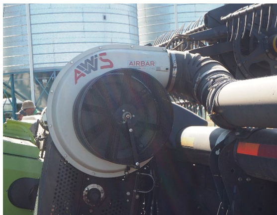
The 'air assist' fitted to the header. Air from the fan (left) is delivered by the multiple silvery pipes (right) which blow grain from shattering seed pods, as they are harvested, on to the header conveyor so it doesn't fall to the ground.
