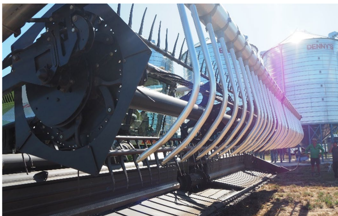
The 'air assist' fitted to the header. Air from the fan (left) is delivered by the multiple silvery pipes (right) which blow grain from shattering seed pods, as they are harvested, on to the header conveyor so it doesn't fall to the ground.
