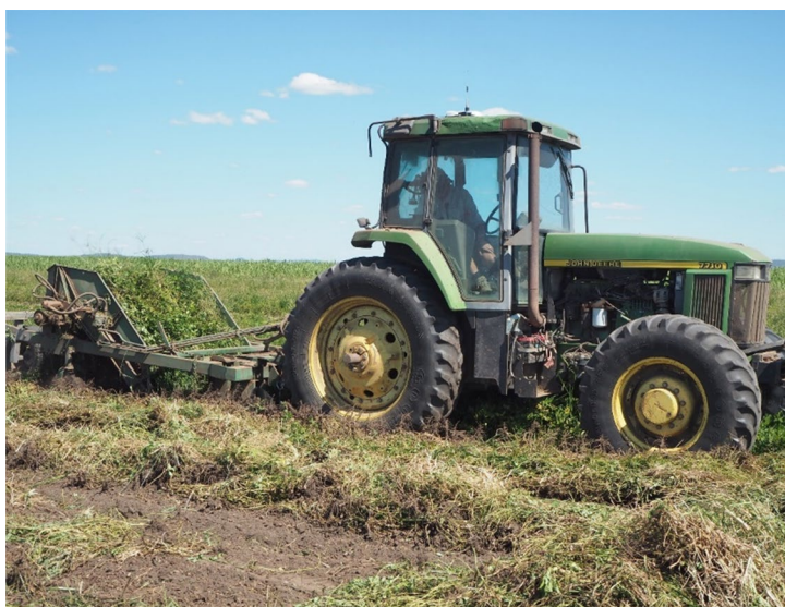
Peanut crop prior to and during digging. The digger has a couple of sharp disks either side of the bed to sever roots and vines growing into the interrow, two horizontal cutter bars arranged in a shallow 'V' that travel under the peanut plants and lift them, and a moving mesh train that lifts the plants allowing some of the soil to fall off. On the downward train are two plates that up-end the plants so the nuts can dry quicker.
