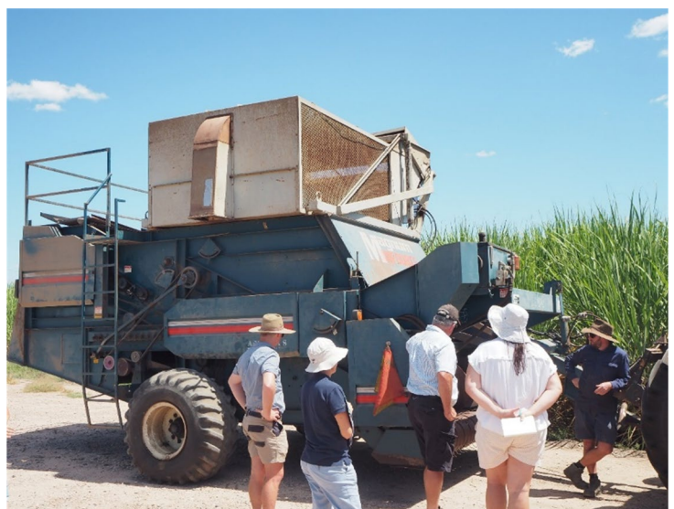
The peanut thresher operated by Aaron Linton. This machine harvests the peanut plants from windrows in the field after they have been dug and partially dried out.
