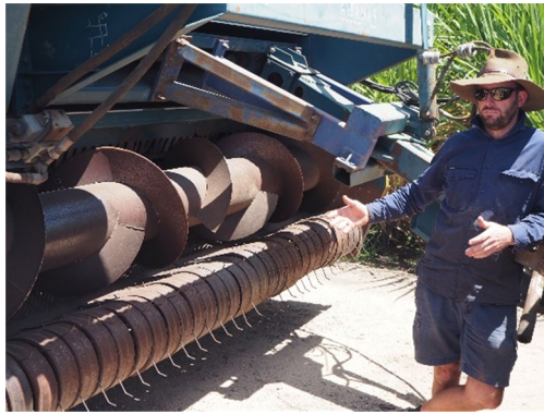
Aaron Linton showing the arrangement on the thresher that lifts the pineapple plants from their windrows once they are sufficiently dry. After lifting, the thresher teases the plants apart, separates the nuts from the rest of the plant and winnows out the leaves and stems.
