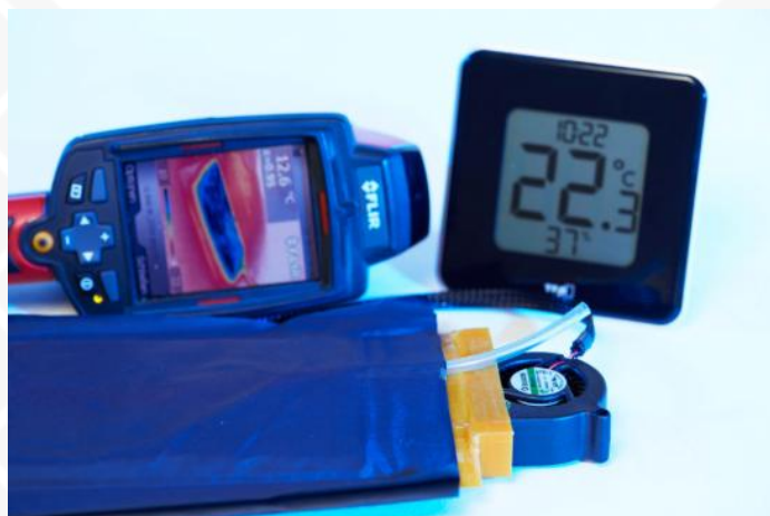
Figure 2: Demonstration of a cooling textile in action, linked to a temperature monitoring device, clearly displaying the real-time temperature of the object undergoing cooling. Image courtesy of ITP GmbH, Germany.
