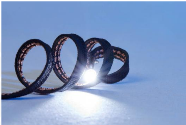
Figure 2: The image shows an advanced smart textile component used in smart textile development. It is more flexible and more durable under bending, which makes it better suited for reliable data and energy transmission in wearables, in comparison with traditional materials used (such as wires and stranded cables). Image courtesy of ITP GmbH, Germany.
