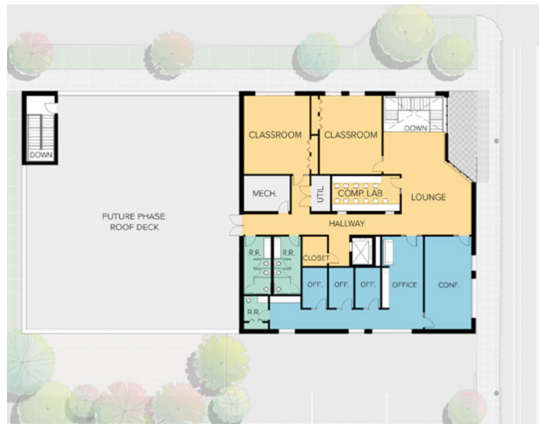
SECOND FLOOR PLAN
