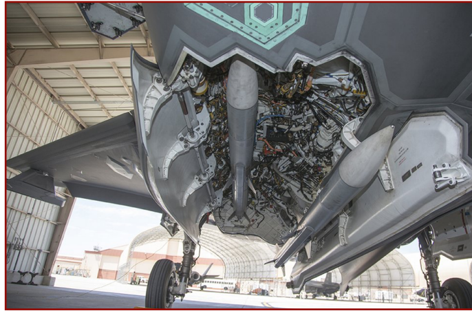
Figure 2: A close-up view of an F-35's internal weapons bay. Weapons bay adapters enable the aircraft to carry a range of munitions, including 1,000-lb GBU-32 bombs, within this compartment. 65
