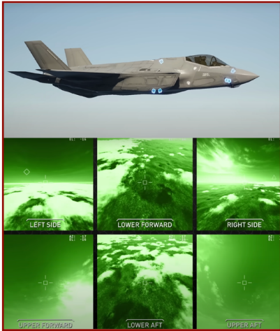
Figure 1: Six highlighted Electro-Optical DAS infrared cameras positioned around the F-35 (top) and the surveillance footage they capture (bottom). 64
